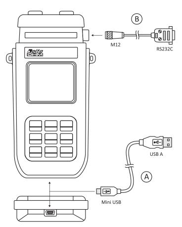
A The HD37AB1347 uses a new serial miniUSB port HD type (Human Interface Device). It is not necessary to install any driver for making the connection to the PC with the USB cable type A – MiniUSB type B coded CP23.
