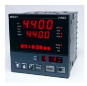
The West 4400 is a powerful Programmer, packed with innovative features to control complex processes. Metal treatment and environmental chambers are typical applications for the 4400.
