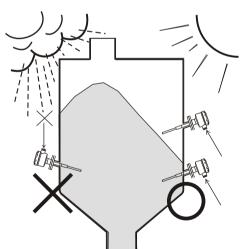
The cable inlet should face downward to avoid rain damage. Tighten the cable with the connecting part.
