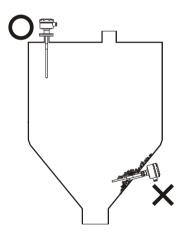
Mounting the probe at top of tank can avoid material bridges from forming. It's helpful to record accurate measurements.
