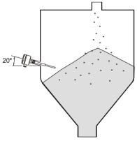
Mounting the probe at a 20° incline will optimize the results and increase sensitivity. It also won't be damaged by the inflowing material.
