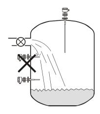
The probe should not be mounted underneath a liquid inlet, otherwise it will switch on erroneously.
