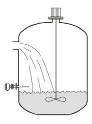
If the tank equips with agitator, please use the time-delay type to prevent fault level detection.
