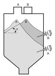
The insensible portion should be mounted to protrude 30mm from the vessel wall. That's to prevent malfunction from a fill material or an insufficient clearance between probe and connection pipe.
