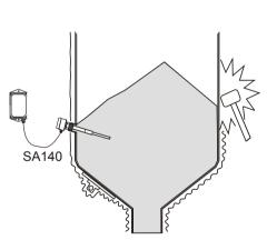
For Non-Stationary or vibrating environment, a separate control unit such as the SA140 is suggested.
