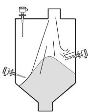
It is suggested to install the probe away from the inlet to reduce the risk of inflowing material damaging the probe. If the probe is near an inlet, it is recommended to place a protective cover 200mm above the probe. The cover should be parallel to the probe and the same length.
