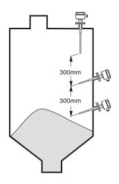
If two parallel probes are mounted, they must be installed separately at least 300 mm to minimize interference .
