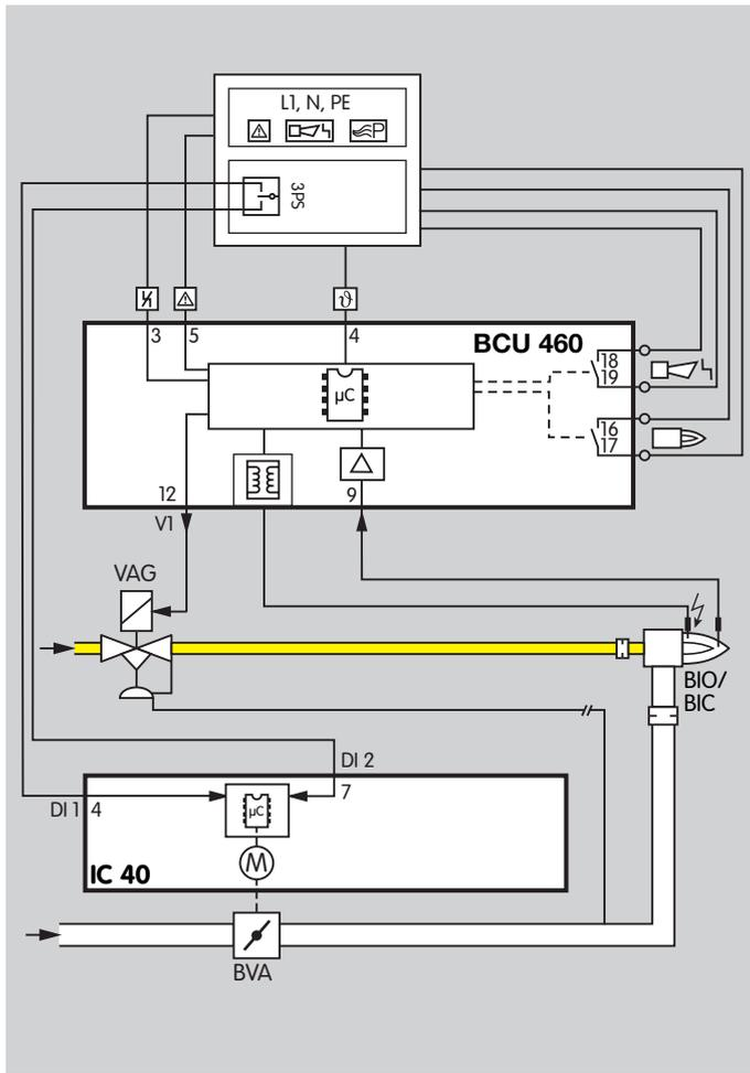
**IC 40, continuous control by three-point step signal.**
