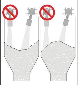
**Liquids Installation Recommendations**Avoid installations where vessel obstructions or fill lines interfere with beam path.
